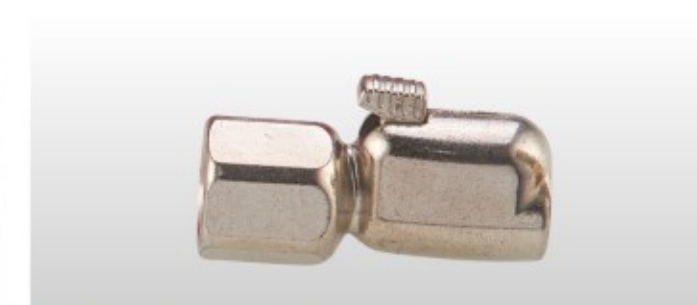
CY-129-2 Tyre inflation nozzle Product: Material: Zinc alloy, aluminum alloy, with rotating function, connector is NPT1/4 or G1/4.
